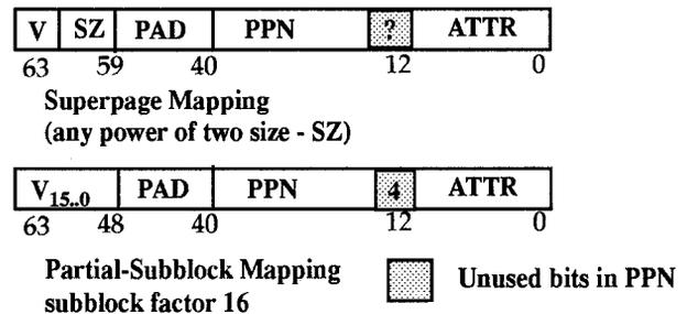
Figure 6: Superpage and Partial-subblock mapping format
