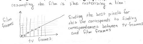
b) [5 pnts] Suggest an appropriate line-drawing algorithm, and fill in the film frames using this algorithm:
