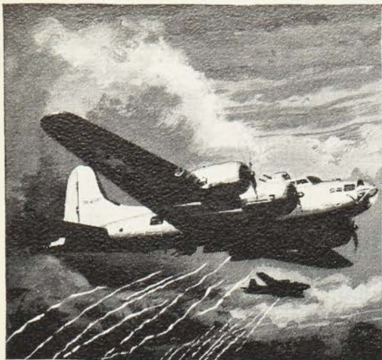
1942 First effective radar countermeasure was "Window," code name for thin strips of metal foil which reflected spurious radar echoes when dropped from Allied bombers, confusing enemy radar operator.
